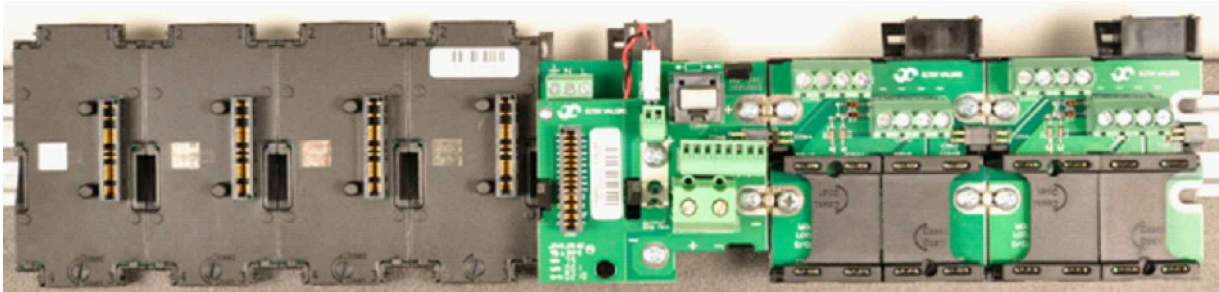
EXAMPLE 3: 4-POSITION BACKPLANE WITH BULK DISTRIBUTION MODULE AND 2 LOAD MODULES (SHOWN WITHOUT COVERS)
