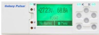
The Pulsar Plus family of controllers provides system monitoring and control features for Infinity, CP, and other power systems. These controllers monitor and control system components including rectifiers, converters, and distribution modules via a multi-drop RS485 digital communications bus. System status, parameters, settings, and alarm
